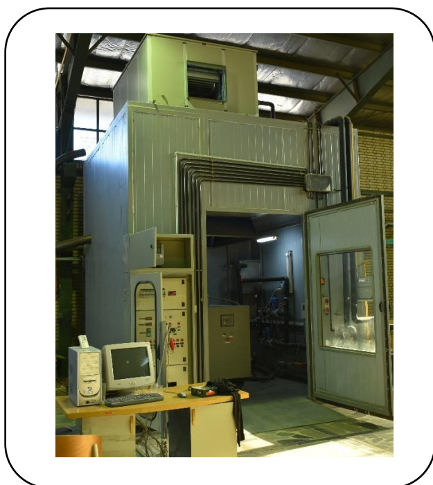
Fig. 2: The manufactured test room with the air handling unit.
