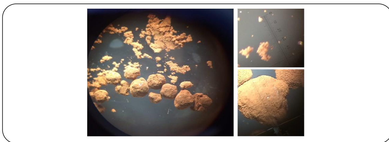
Fig. 6: The grain size of the gold recovered at different aqueous SO 2 solution volumes.
