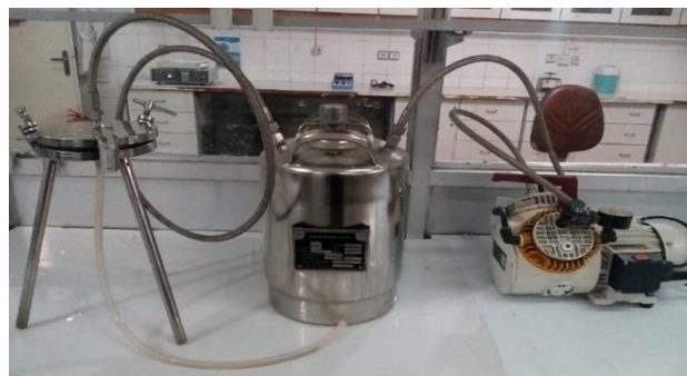
Fig. 1: filter Press system, including transfer pump, storage tank, and membrane holder
