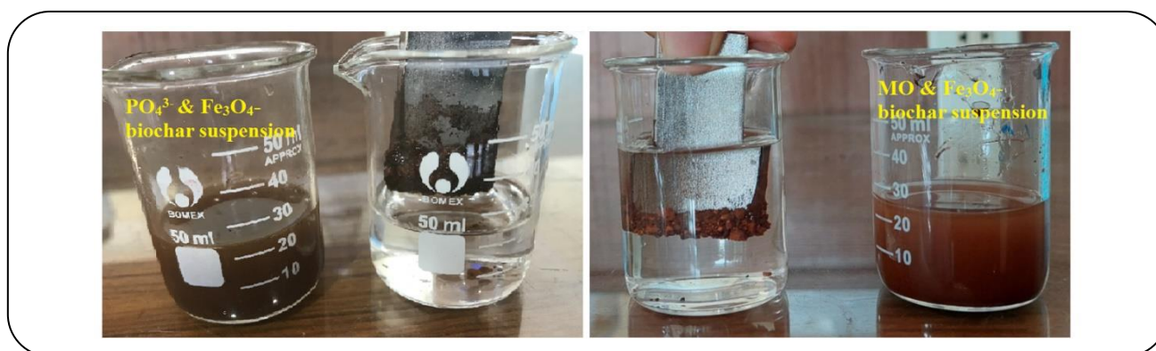
Fig. 8: \text{Fe}_3\text{O}_4 -biochar collected \text{PO}_4^{3-} or MO from the suspension by a magnet.
