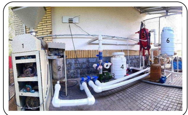
Fig. 1: Schematic diagram of the process: Extruder (1); Mixer (2); Pump (3); Homogenizer tank (4); digester (5); Storage tank (6).
