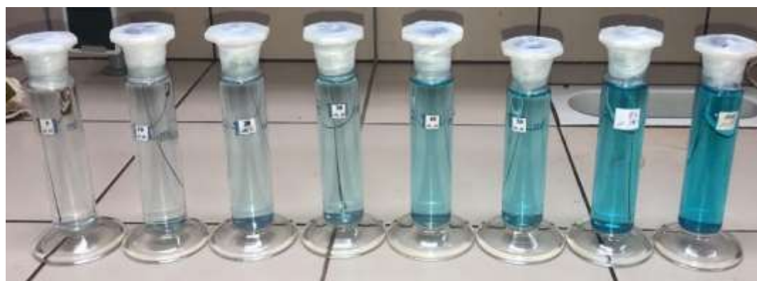
Fig. 1: Color change of solution in oxygen measurement using the colorimetric method
