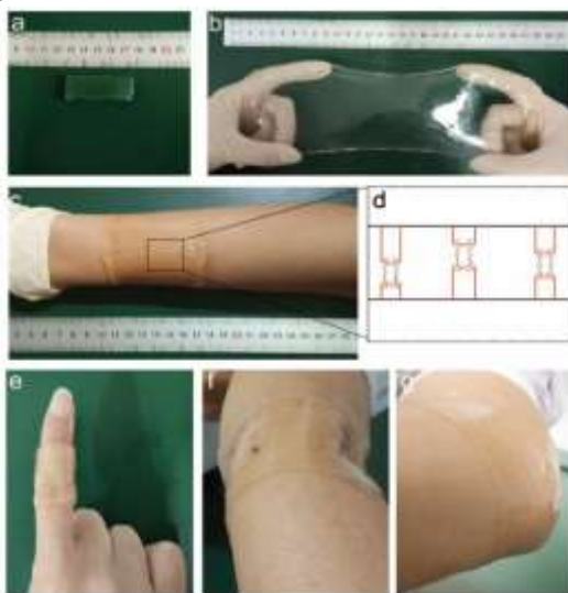
Fig. 5: Adhesion properties of PAM-Ag + hydrogels in medical dressing.
