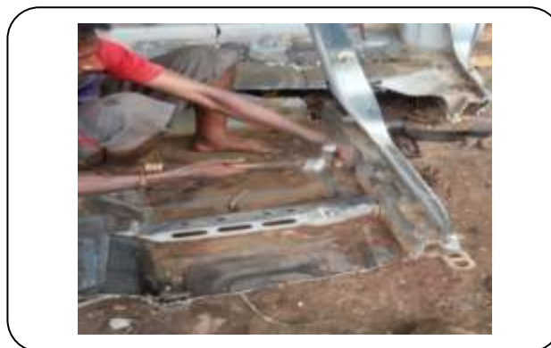
Fig. 5: Usage of inefficient tools - Breaking the car body with a hammer.
