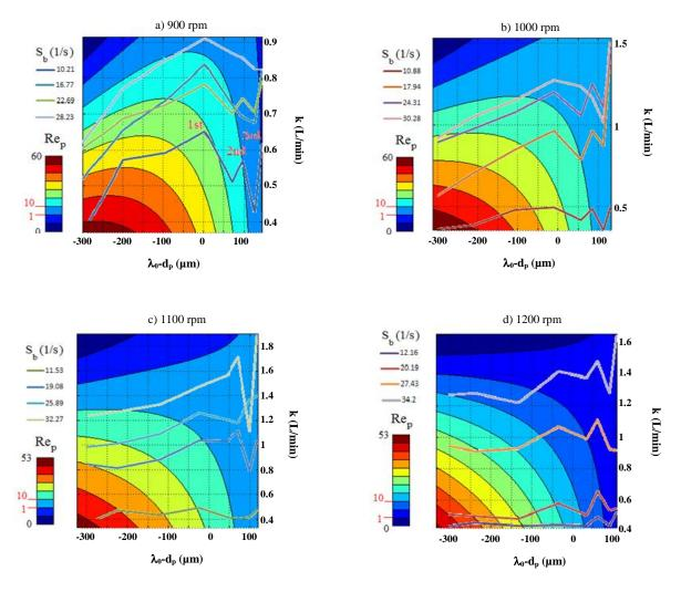
Fig. 8: The effect of particle Reynolds number on the k-S<sub>b</sub> relationship.
