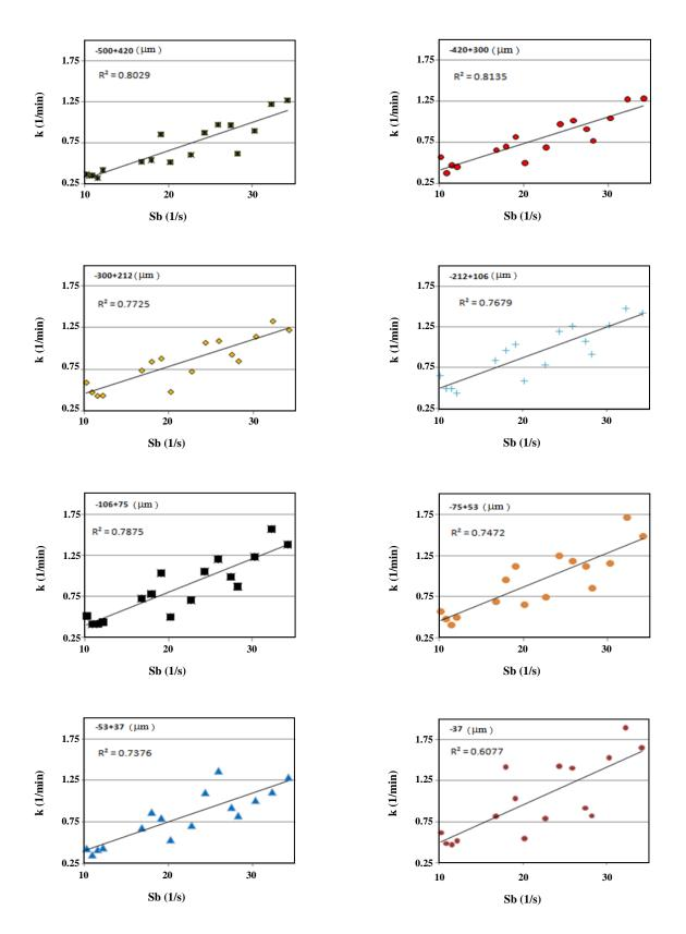
Fig. 2: k-S<sub>b</sub> relationship for different particle sizes.
