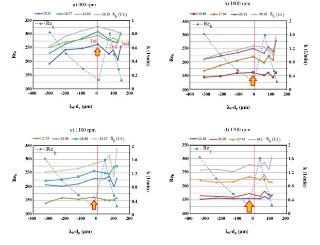
Fig. 4: The Effect of micro turbulence and bubble Reynolds number on the k-S<sub>b</sub> relationship.
