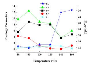
Fig. 2: Effect of temperature on reheology property of MSP modified drilling fluids.
