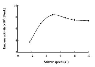
Fig. 3: Effect of stirrer speed on extraction of lipxygenase-1.
