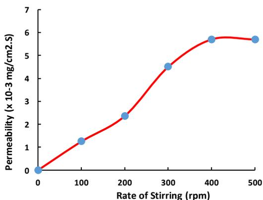
**Fig. 5: Effect of stirring speed (volume of source phase 260 mL of 50mg/L of dye at pH 7 ± 0.1, carrier concentration 4.48 × 10<sup>-1</sup> mol/L, volume of receiving phase 260 mL of 1N H<sub>2</sub>SO<sub>4</sub>, and effect of time 70 min).**
