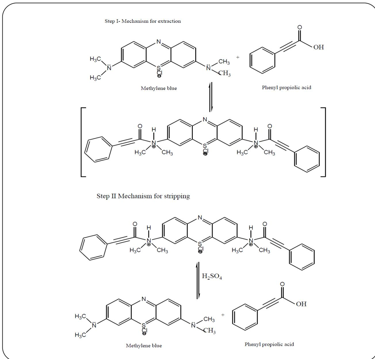
**Fig. 9: Extraction and stripping mechanism for MB.**
