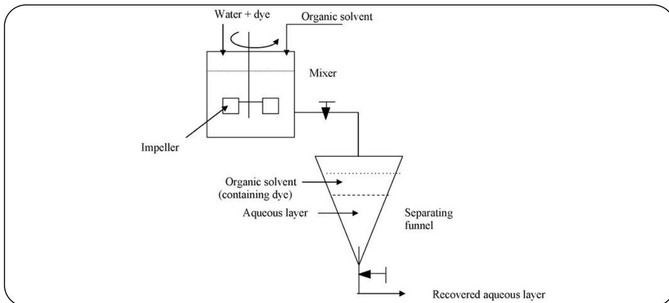
Fig. 1: Schematic experimental setup for liquid-liquid extraction for removal of dye from aqueous solution.
