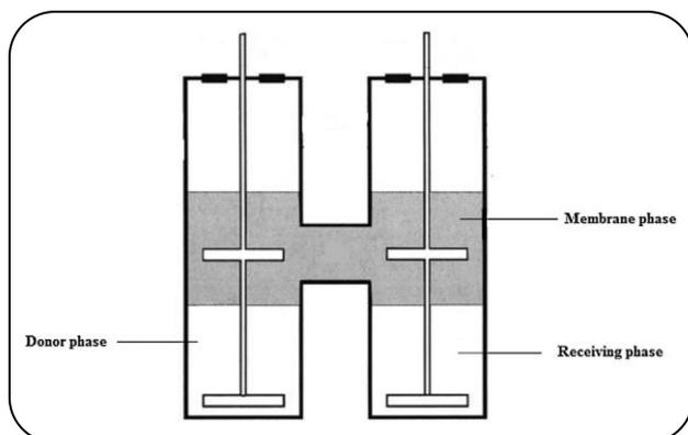
Fig. 2: Schematic experimental setup for bulk liquid membrane for transport of dye from aqueous solution.
