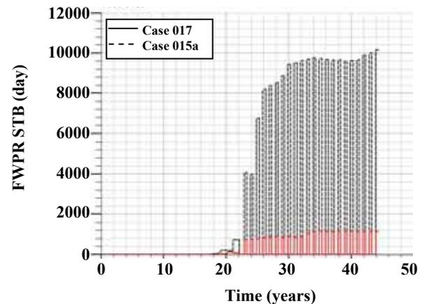
Fig. 13: Water production in reservoir with vertical wells (case 015a) and horizontal wells (case 017) Table 1-Initial reservoir fluid composition.
