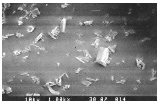
Fig. 10: Aluminum fluoride crystals after 270 minutes of crystallization.
