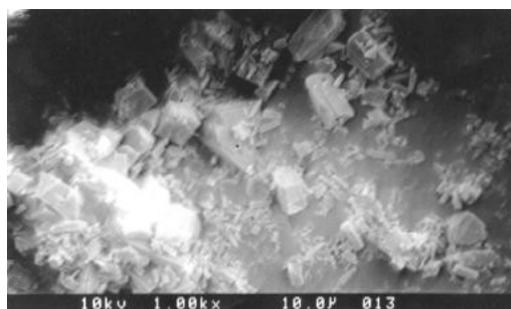
Fig. 9: Aluminium fluoride crystals after 210 minutes of crystallization.
