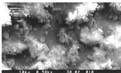
Fig. 8: Aluminum fluoride crystals after 150 minutes of crystallization.
