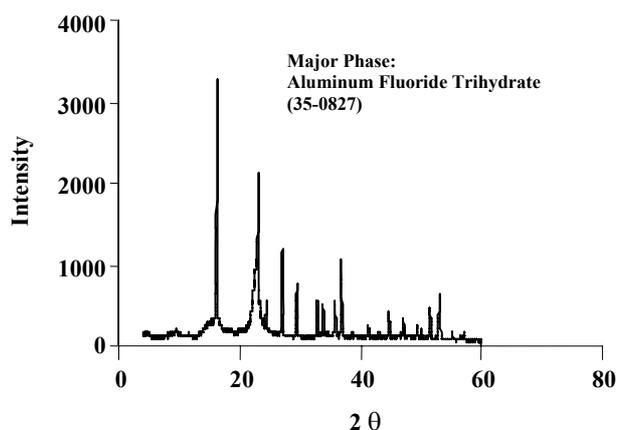
Fig. 3: XRD analysis from crystals of sample 2.
