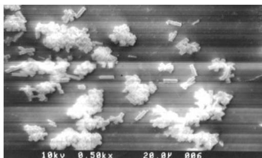
Fig. 7: Aluminum fluoride crystals after 75 minutes of crystallization.
