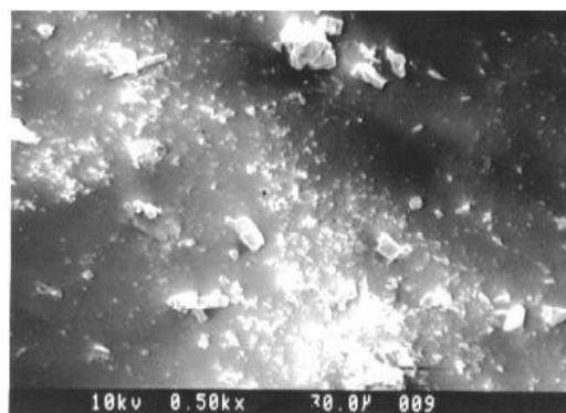
Fig. 6: Aluminum fluoride crystals after 45 minutes of crystallization.
