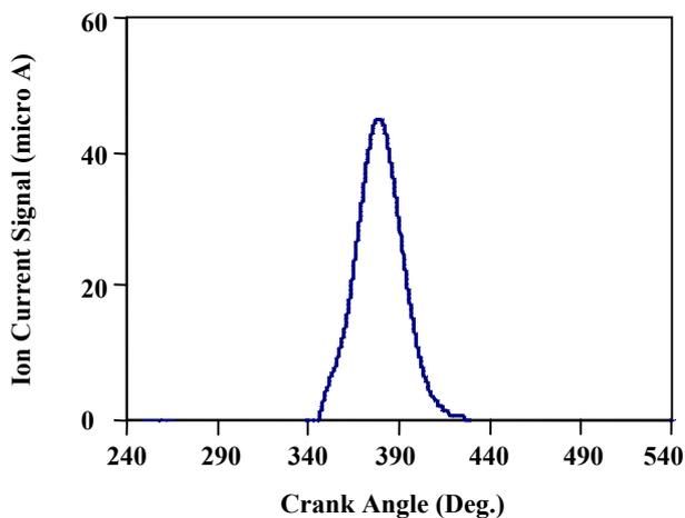
Fig. 8: Ion current variation in post flame period (Simulated).
