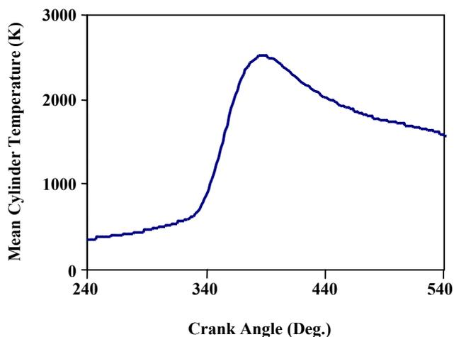
Fig. 5: Mean cylinder temperature verses crank angle (Simulated).
