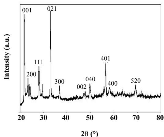
Fig. 5. XRD pattern of  $WO_3$  film fired at 500 °C.
