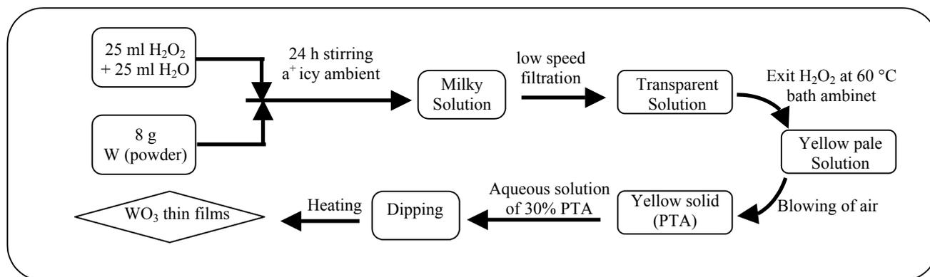
Fig. 1: The various films processing steps in  $WO_3$  preparation.
