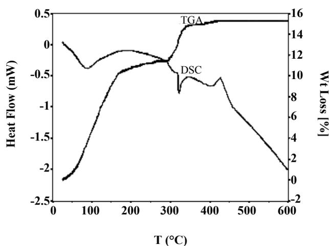
Fig. 4: TGA-DSC patterns of xerogel.
