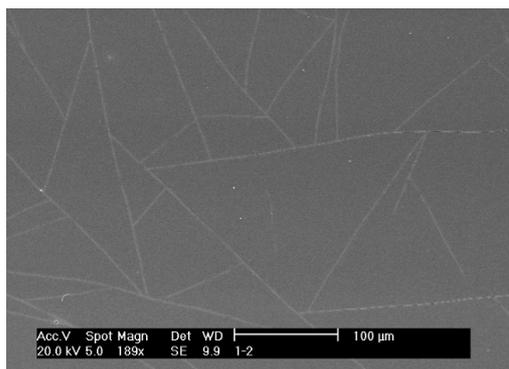
**Fig. 7:** Scanning electron micrograph of  $WO_3$  film deposited on ITO glass substrate, annealed at  $200^\circ C$ .
