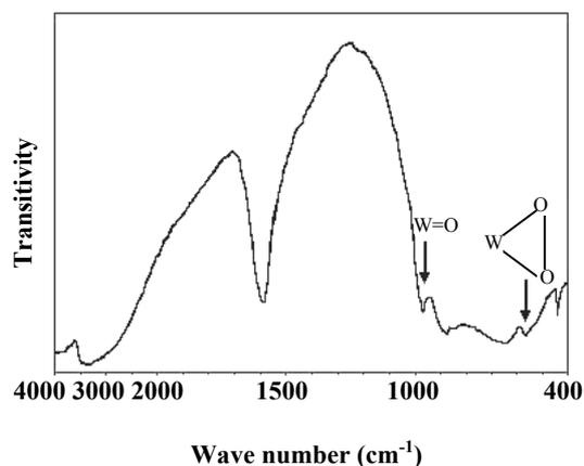
Fig. 2: FT-IR Spectra for  $WO_3$  film (KBr tablet).
