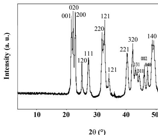
Fig. 3: XRD pattern of  $WO_3$  powder calcinated at  $500^\circ C$ .
