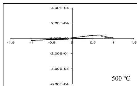
Fig. 6. Cyclic voltammograms of  $WO_3$  films on ITO glass electrode in 1M  $H^+$  solution, fired at different temperatures.
