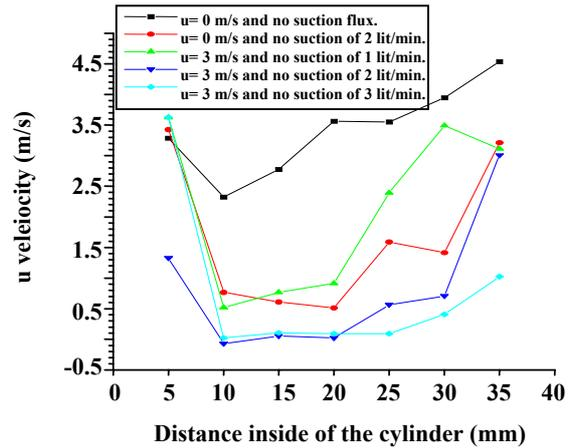
Fig. 5: Centre-line  $u$  velocities measured inside of a sampler (20 mm front orifice, 4 mm back orifice) for different conditions.
