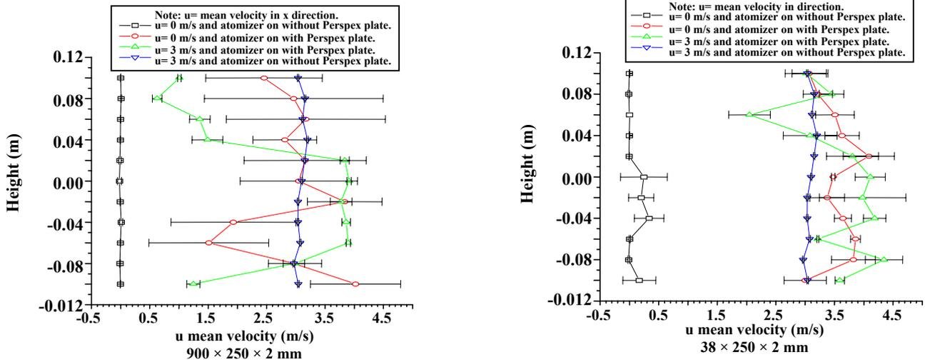
Fig. 8: Centre-line  $u$  velocity, measured at centre of the empty test section for different conditions in the vicinity of two different sizes of perspex plates.
