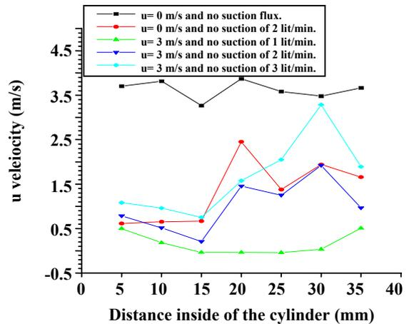
Fig. 6: Centre-line  $u$  velocities measured inside of a sampler (10 mm front orifice, 4mm back orifice) for different conditions.
