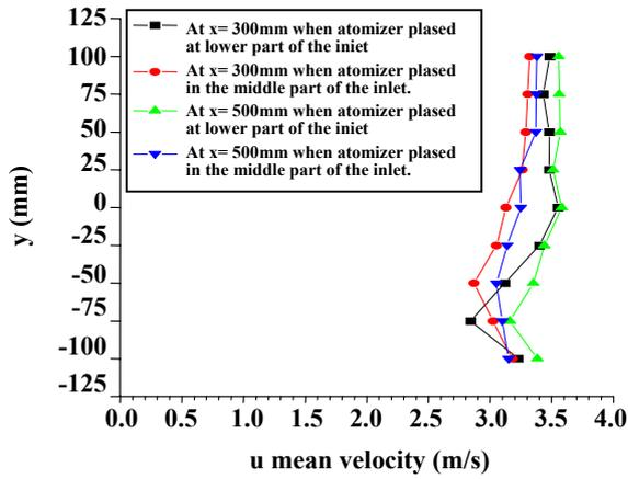
Fig. 2: Centre-line  $u$  mean velocity measurements inside of an empty test section of the wind tunnel when the particle generator is placed at lower and middle part of the inlet at a wind speed of  $U = 3$  m/s.
