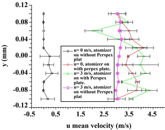
Fig. 3: Centreline  $u$  velocity, measured at centre of the empty test section for different conditions.
