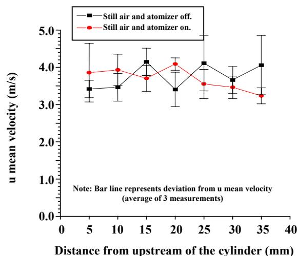
Fig. 12: Centre-line  $u$  mean velocity measurements inside of the metal cylinder ( $38 \times 40$  mm, copper) with 4 mm inlet and outlet orifices and an open slit of  $38 \times 20$  mm when discharged by earthing in still air.
