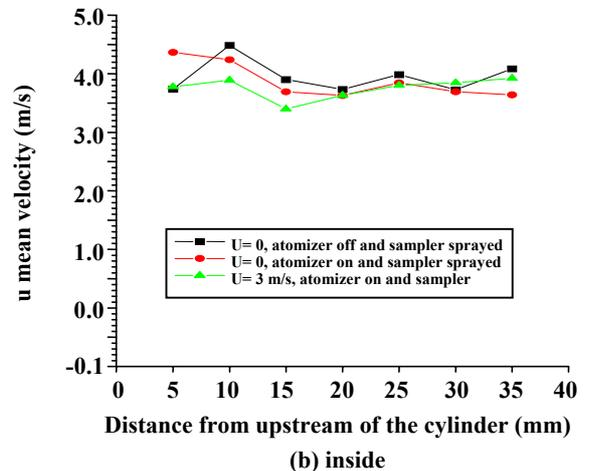
Fig. 9: Centre-line  $u$  mean velocity measurements at (a) upstream and (b) inside of the acrylic sampler (38x40 mm, perspex cylinder) with 4 mm inlet and outlet orifice when sprayed by an anti-electrostatic liquid in still and moving air.
