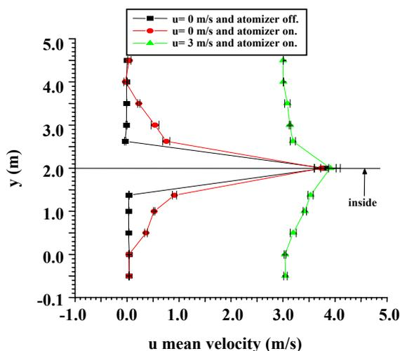
Fig. 11: Cross sectional  $u$  mean velocity measurements at the centre of the metal cylinder ( $38 \times 40$  mm, copper) with 4 mm inlet and outlet orifices and an open slit of  $38 \times 20$  mm at different conditions.
