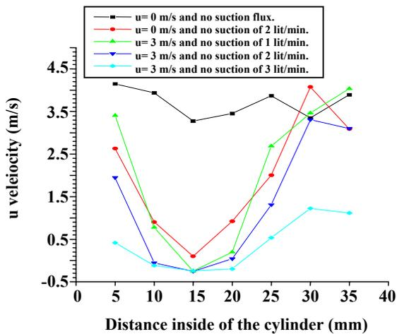
Fig. 4: Centre-line  $u$  velocities measured inside of a sampler (front fully open, 4 mm back orifice) for different conditions.
