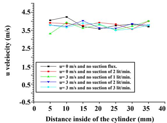
Fig. 7: Centre-line  $u$  velocities measured inside of a sampler (4 mm front orifice, 4 mm back orifice) for different conditions.
