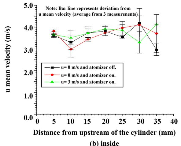
Fig. 10: Centre-line  $u$  mean velocity measurements at (a) upstream and (b) inside of metal cylinder (38x40 mm, copper) with 4 mm inlet and outlet orifices and an open slit of 38x20 mm in still and moving air conditions.
