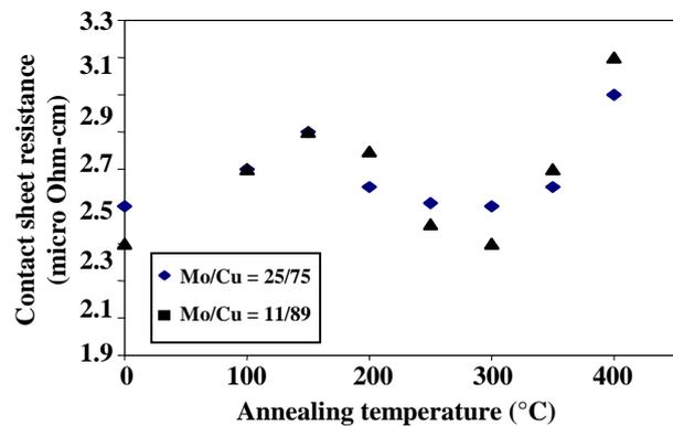
Fig. 9: Contact sheet resistance versus the annealing temperature for Cu-Mo structures with different Mo/Cu thickness ratios. A local minimum sheet resistance can be observed at about 300 °C.
