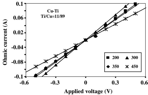
Fig. 6: Total current versus the applied voltage for the ohmic contacts with different annealing temperatures for Cu-Ti structure. An optimum temperature of about 300 °C has been obtained.
