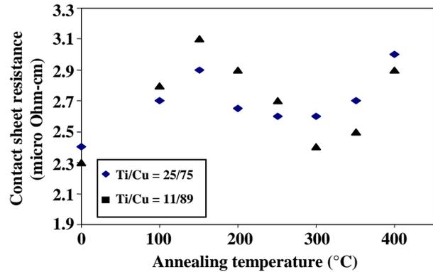
Fig. 8: Contact sheet resistance versus the annealing temperature for Cu-Ti structures with different Ti/Cu thickness ratios. A local minimum sheet resistance can be observed at about 250 °C- 300 °C.
