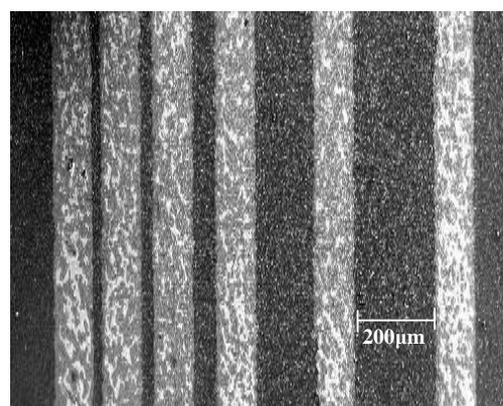
**Fig. 2: SEM image of a sample after the annealing and the lithography process. The metal alloy has been patterned with a mask designed for the realization of the TLM method.**
