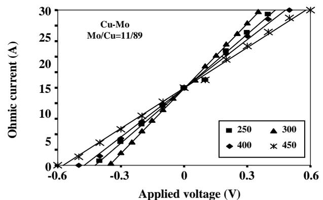
Fig. 5: Total current versus the applied voltage for the ohmic contacts with different annealing temperatures for Cu-Mo structure. An optimum temperature of about 300 °C has been obtained.
