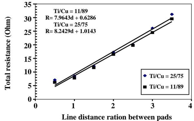
Fig. 3: Variation of the total contact resistance with the distance between TLM lines for two different Ti/Cu thickness ratio annealed at the temperature of 350 °C.  $R_C$  and  $R_{SEM}$  can be extracted from the line equations that have been shown in the of the figure.
