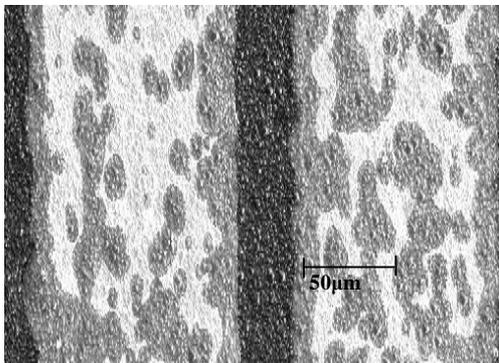
Fig. 7: SEM image of the alloys which have been annealed above 450 °C. As can be seen, due to the high diffusivity of the Cu atoms, Cu has passed Ti or Mo film and has reached to the silicon substrate.
