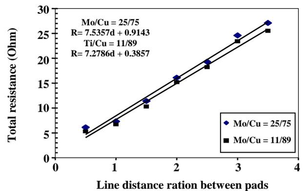
Fig. 4: Variation of the total contact resistance with the distance between TLM lines for two different Mo/Cu thickness ratio annealed at the temperature of 350 °C. As can be seen, Mo has lower resistance than Ti.
