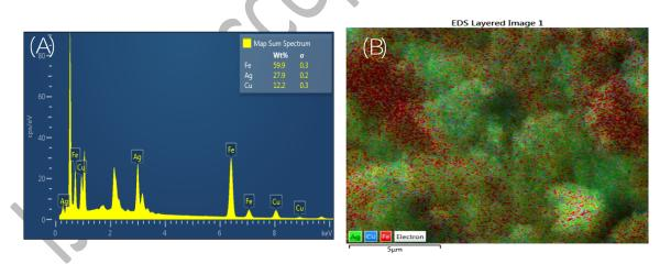
Fig. 3 A) The EDS images of  $Fe_2O_3/Cu/Ag$  Fig. 3 B) the mapping images of  $Fe_2O_3/Cu/Ag$
