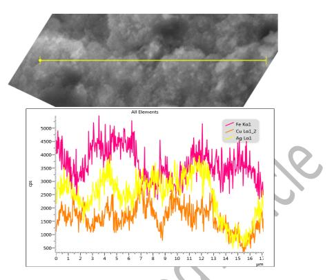
Fig. 4: The EDX line scan analysis for Fe<sub>2</sub>O<sub>3</sub>/Cu/Ag
