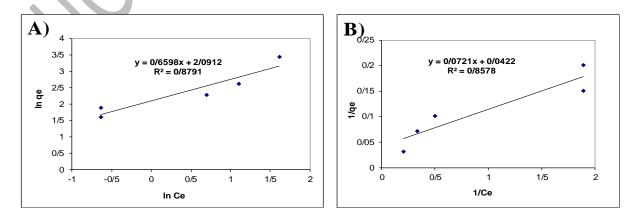
Fig. 9. Freundlich and Langmuir isotherm for tetracycline adsorption on adsorbent at room temperature
