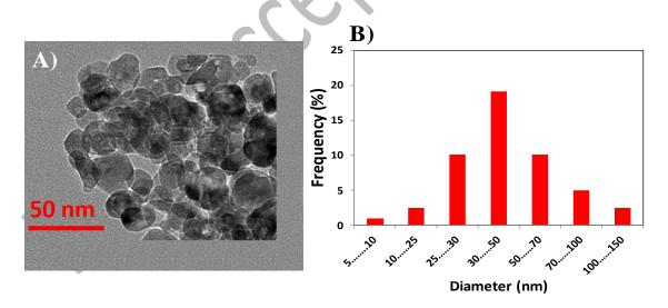
Fig. 5A) The TEM images of Fe<sub>2</sub>O<sub>3</sub>/Cu/Ag, Fig. 5B) histogram for TEM of Fe<sub>2</sub>O<sub>3</sub>/Cu/Ag
