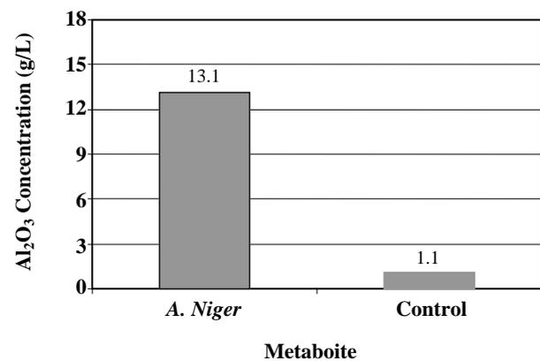
Fig. 7: Concentration of Al<sub>2</sub>O<sub>3</sub> during bioleaching of red mud by *A. Niger* (g/L).
