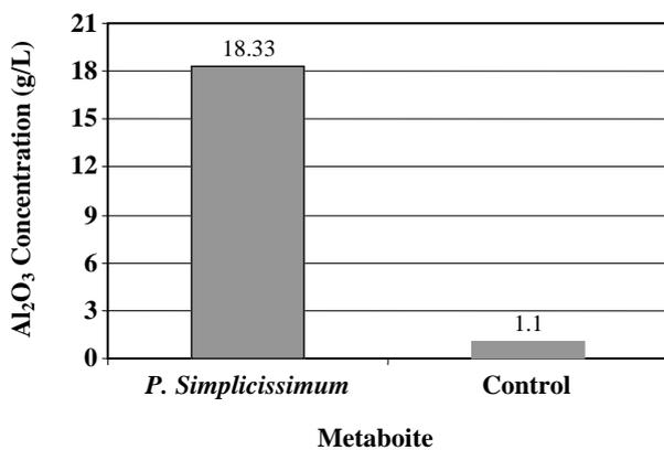
Fig. 6: Concentration of Al<sub>2</sub>O<sub>3</sub> during bioleaching of red mud by *P. Simplicissimum* (g/L).
