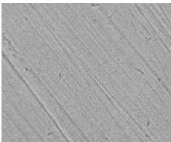
Fig. 6: SEM image of polished MS surface.
