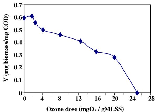
Fig. 7: The effect of Ozone does on Y.
