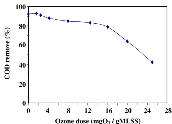
**Fig. 4: The effect of ozone does on COD removal efficiency.****The effect of different ozone doses on SVI**
