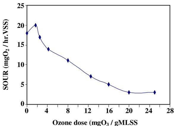
Fig. 6: The effect of Ozone does on SOUR.
