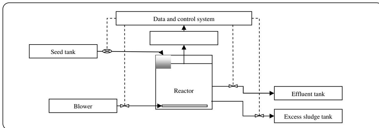
Fig.1: The general view of SBR schematic.
