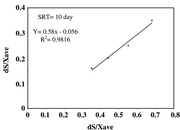
**Fig. 3: Determination of Y and  $k_4$  in SRT =10 days. Under no-ozone-addition condition.****The effects of different ozone doses on COD removal co-efficiency**
