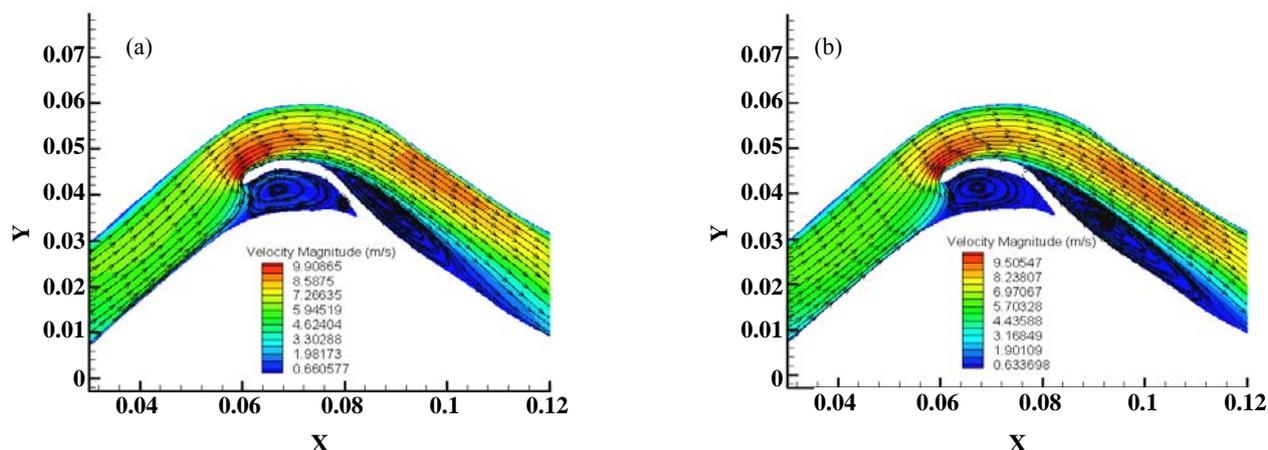
Fig. 6: The stream traces and velocity magnitude contours at the bulk air velocity of 3.54 m/s obtained by:
