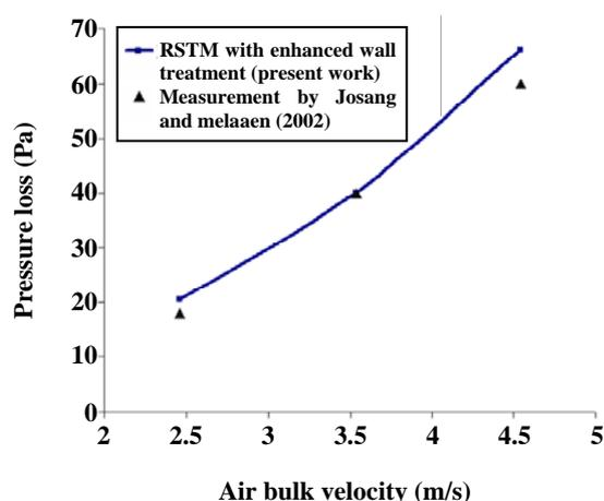
**Fig. 9: The calculated pressure loss versus the air bulk velocity for 25mm plate spacing.**
