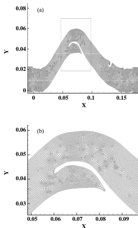
Fig. 5: Unstructured mesh generated for gas flow computation a) whole mesh b) details of mesh at bend.
