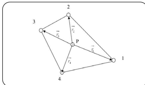
**Fig. 3: Droplet location at a computational air field cell (point P).**
