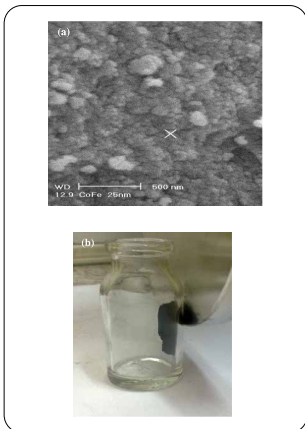
Fig. 1: (a) SEM image of \text{CoFe}_2\text{O}_4 magnetic nanoparticles, (b) photograph showing magnetic property of \text{CoFe}_2\text{O}_4 nanoparticles.
