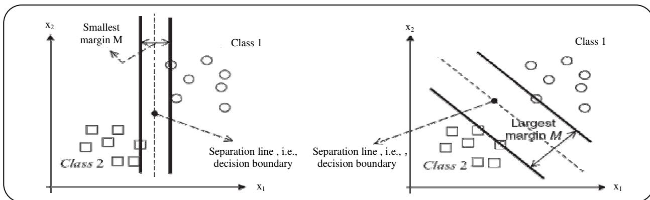
**Fig. 4:** This figure demonstrates two different separating lines with different margins for a set of training data. It is obvious that the line in the right figure provides a wider margin than the left one and thus is more desirable. (Photo taken from [38]).
