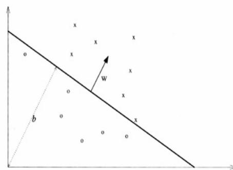
Fig. 3: A linear classifier which separates two classes of training data. Vectors  $b$  and  $w$  are visualized in this picture. Photo taken from [37].
