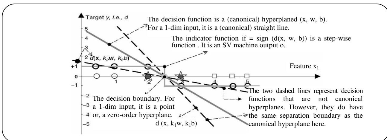
**Fig. 5:** This photo demonstrates the difference between canonical separating line and other separating files. (Photo taken from [38]).
