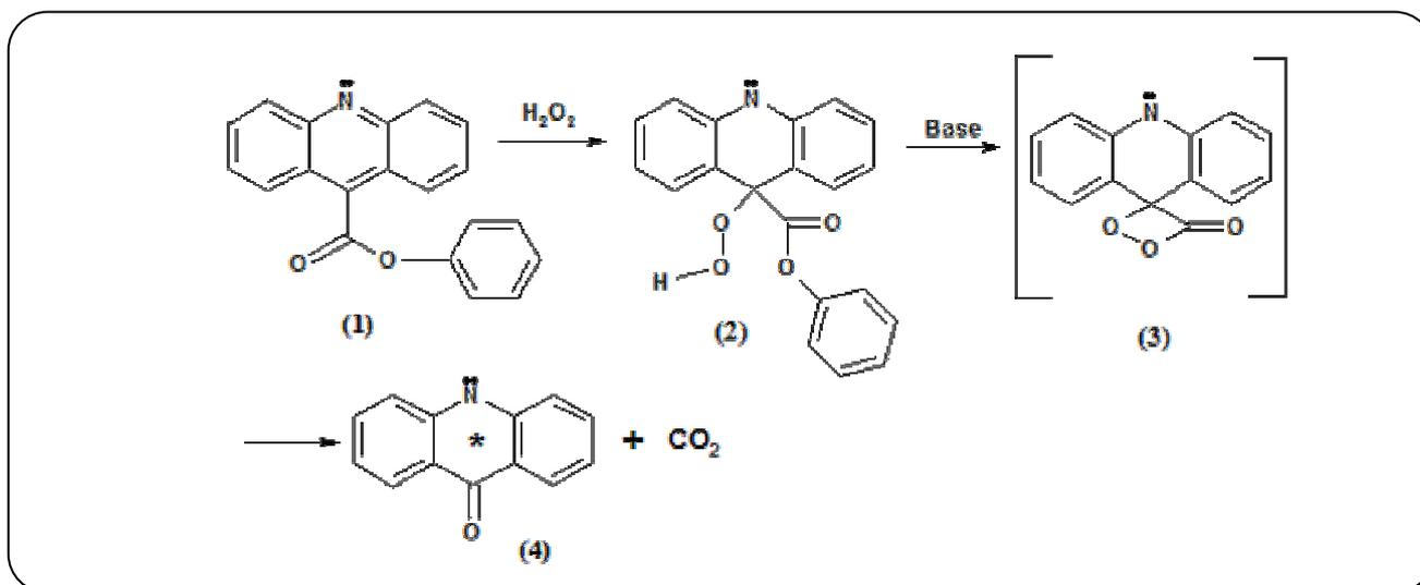
Fig. 1: Mechanism of the CL of acridinium esters.
