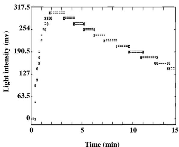
Fig. 11: A typical computer fit of the CL intensity time plot for the acridinium ester - $\text{H}_2\text{O}_2$  -Rhodamin B system according to the data of luminometric measurements. The acridinium ester concentration is  $2 \times 10^{-6} \text{ mol L}^{-1}$ . (x) experimental point; (o) calculated point; (=) experimental and calculated points are the same within the resolution of plot.
