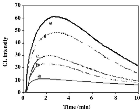
Fig. 6 : CL intensity as a function of time for reaction of acridinium ester ( $5 \times 10^{-3} \text{ mol L}^{-1}$ ) with varying concentration of  $\text{H}_2\text{O}_2$  in the presence of rhodamin B ( $1 \times 10^{-4} \text{ mol L}^{-1}$ ) in methanol: (a)  $0.58 \times 10^{-3}$ , (b)  $1.16 \times 10^{-3}$ , (c)  $1.17 \times 10^{-3}$ , (d)  $2.32 \times 10^{-3}$ , (e)  $2.91 \times 10^{-3} \text{ mol L}^{-1}$ .
