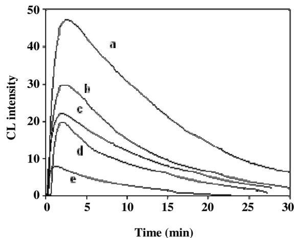
Fig. 4: CL intensity of time for reaction of acridinium ester ( $5 \times 10^{-3} \text{ mol L}^{-1}$ ) with  $\text{H}_2\text{O}_2$  (35%) in the presence of rhodamin B ( $1 \times 10^{-4} \text{ mol L}^{-1}$ ) and varying concentration of sodium hydroxide in acetone/water 70/30 (v/v) solutions: (a)  $10 \times 10^{-6}$ , (b)  $20 \times 10^{-6}$ , (c)  $40 \times 10^{-6}$ , (d)  $60 \times 10^{-6}$ , (e)  $80 \times 10^{-6} \text{ mol L}^{-1}$ .
