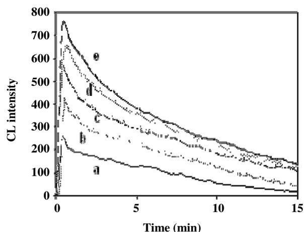
Fig. 8: The CL intensity as a function of time for reaction of varying concentration of lucigenin with  $\text{H}_2\text{O}_2$  (35%) in the presence of triethyl amine ( $0.1 \text{ mol L}^{-1}$ ) in acetone/water (70/30 v/v) as a solvent by a home-made luminometer: (a)  $1.82 \times 10^{-7}$ , (b)  $3.64 \times 10^{-7}$ , (c)  $5.45 \times 10^{-7}$ , (d)  $7.27 \times 10^{-7}$ , (e)  $9.1 \times 10^{-7} \text{ mol L}^{-1}$ .
