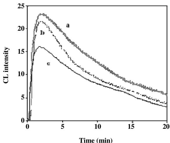
Fig. 10 : The CL intensity as a function of time for reaction of varying concentration of rhodamin B (a-c:  $0.1 \times 10^{-7}$ - $0.3 \times 10^{-7} \text{ mol L}^{-1}$ ) in methanol for 100-300  $\mu\text{L}$  injection.
