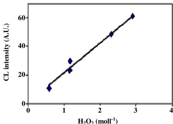
Fig. 12: Effect of  $H_2O_2$  concentration ( $10^{-3} \text{ mol L}^{-1}$ ) on the CL intensity of acridinium ester - $H_2O_2$  -Rhodamin B system in the presence of ( $0.4 \text{ mol L}^{-1}$ ) sodium hydroxide.  $Y=20.837x+0.8283$ ,  $R^2=0.9821$ .
