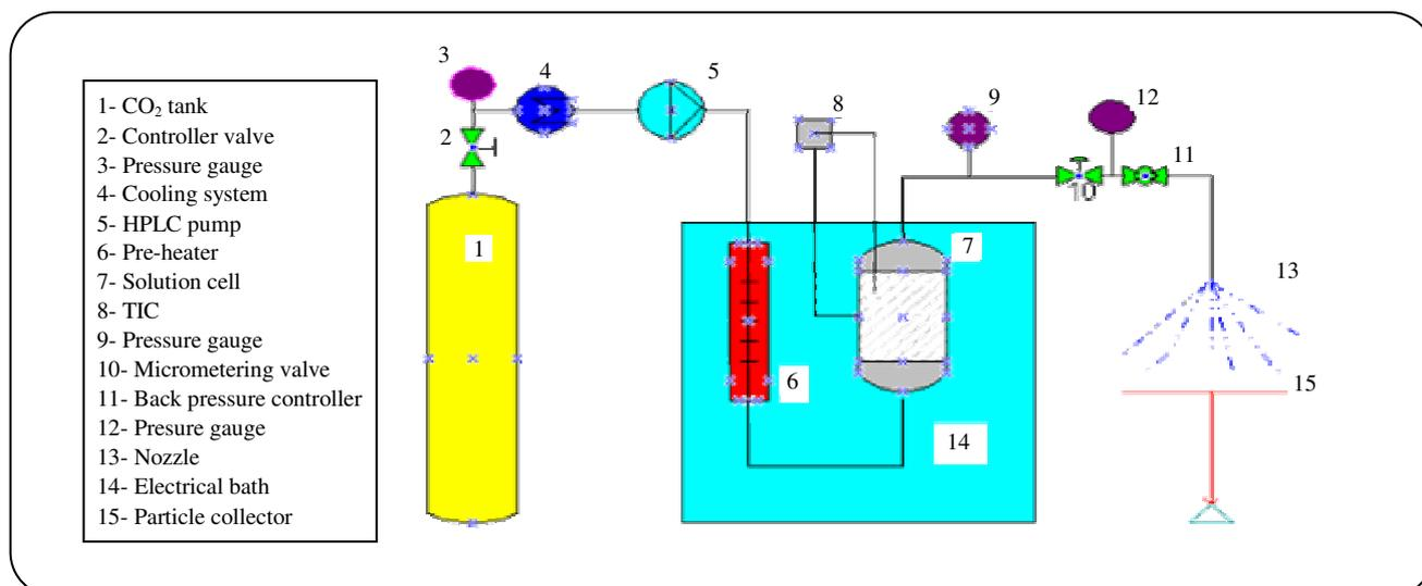
Fig. 1: RESS Apparatus.
