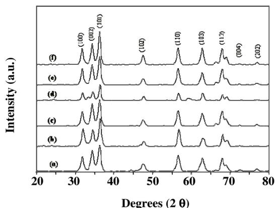
Fig. 2: XRD patterns of synthesized samples: (a) ZnO-5, (b) ZnO-15, (c) ZnO-20, (d) ZnO-25, (e) ZnO-20a, (f) ZnO-20b.
