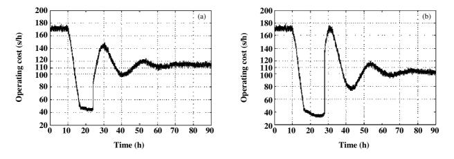
Fig. 3: Cost functions obtained by (a) crisp RTO, and (b) fuzzy RTO.
