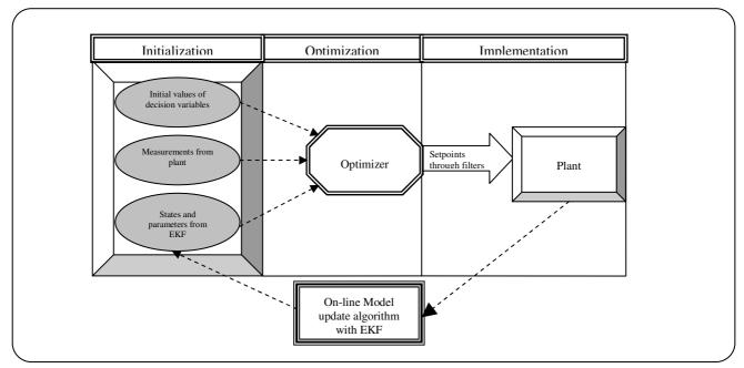
Fig. 2: Schematic diagram of the RTO algorithm.
