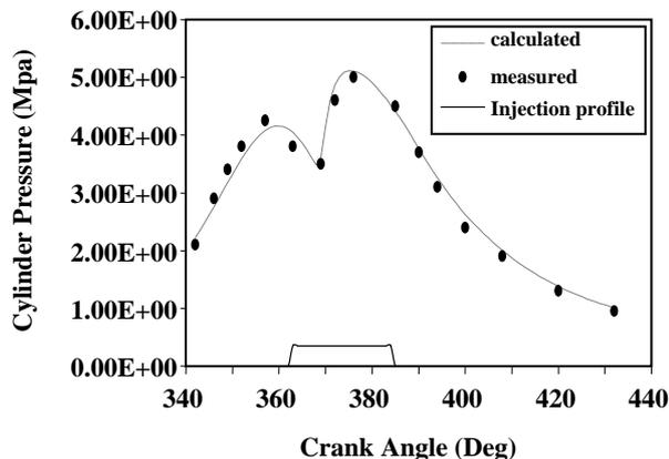
Fig. 2: Comparison of calculated and measured [8] in-cylinder pressure.
