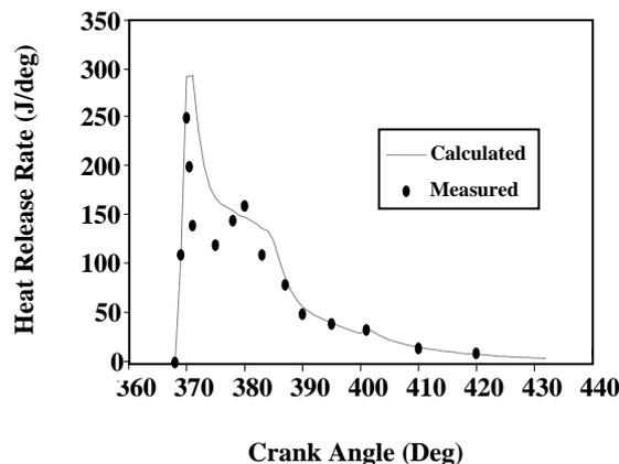
Fig. 3: Comparison of calculated and measured [8] heat release rate.
