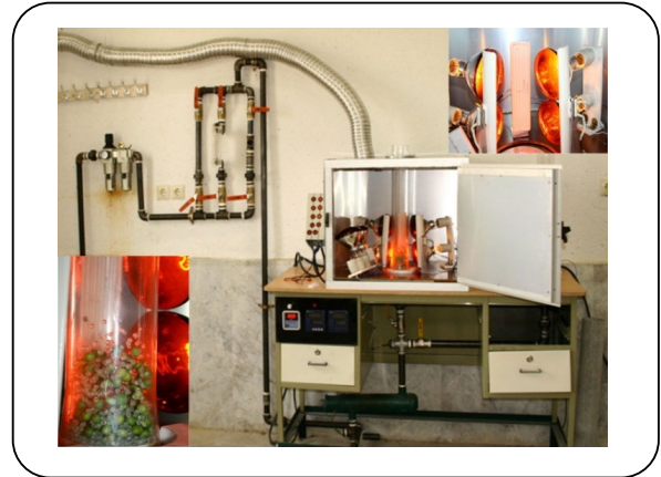
Fig. 2: Fluidized Bed Dryer (FBD) assisted by infrared heating set up.
