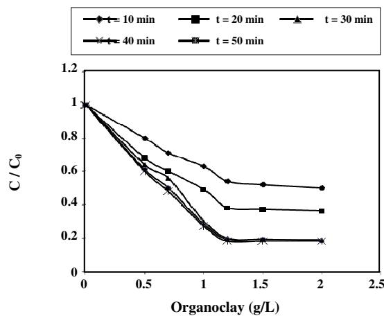
Fig. 7: Organoclay concentration on pollution adsorption at pH=4.5.
