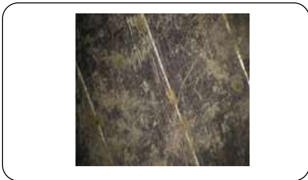
Fig. 6: Traces of contact of the media with the surface of steel 45 after 20 min before treatment (x 15)
