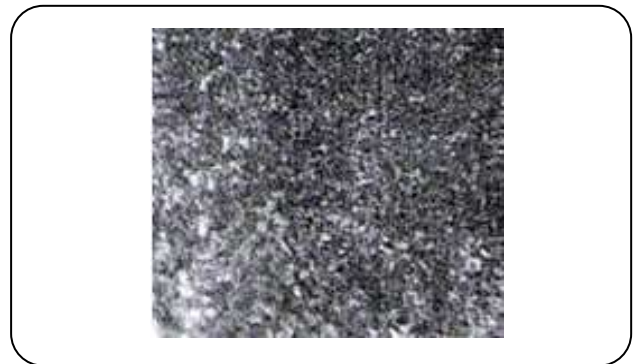
Fig. 7: Traces of contact of the media with the surface of steel 45 after treatment.
