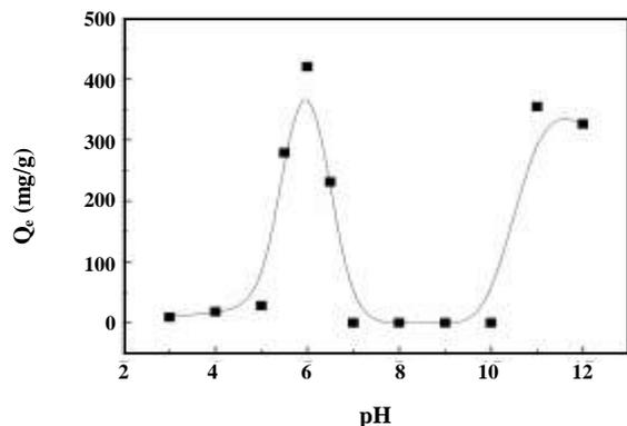
Fig. 4: Effect of pH on the uptake of Pb(II) at different pH values (3-12).
