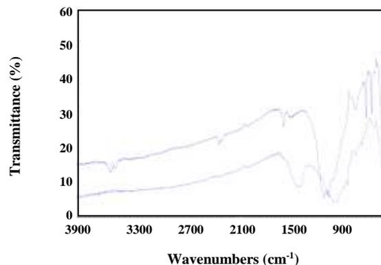
Fig. 1: FT-IR spectra of MB and Pb(II)-loaded MB.
