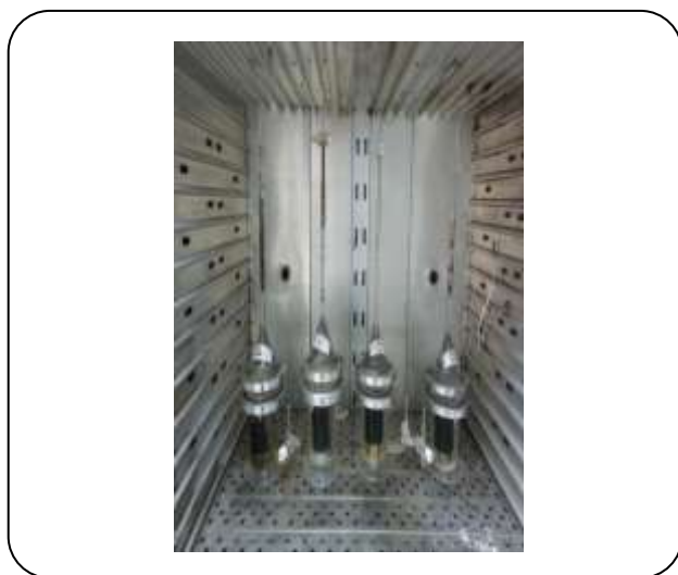
Fig. 2: (a) The oil recovery percentages for four core samples during 30 days without any nanoparticles (b) Amott cell in the last day.
