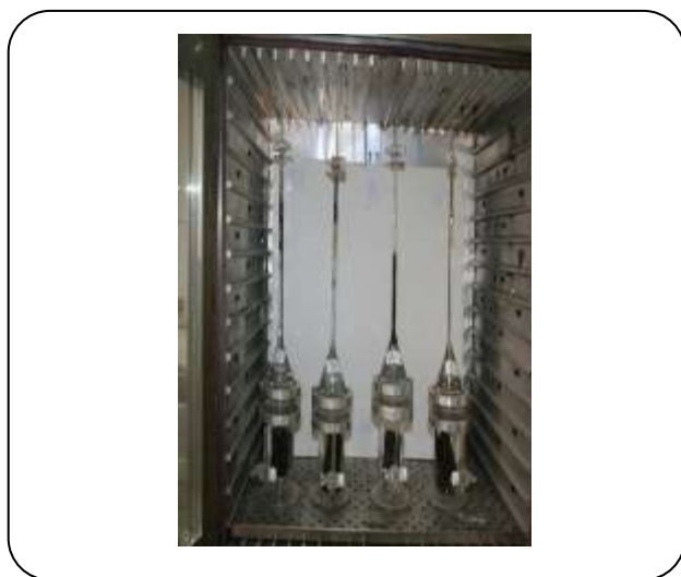
Fig. 3: (a) The oil recovery percentages for four core samples during 30 days with CuO nanoparticles (b) Amott cell in the last day.
