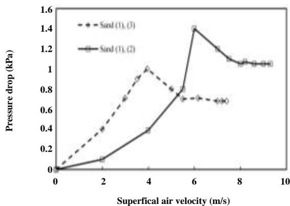
Fig. 7: Effect of particles diameter on pressure drop in spouted bed containing binary mixture for static bed height,  $h = 20$  cm, and cone angle  $= 30^\circ$ . (Flotsam rich: sand (1): 1.77mm, 2650 kg/m<sup>3</sup>, 5%; sand (2): 0.575 mm, 2650 kg/m<sup>3</sup>, 95%; sand (3): 0.356 mm, 2650 kg/m<sup>3</sup>, 95%).
