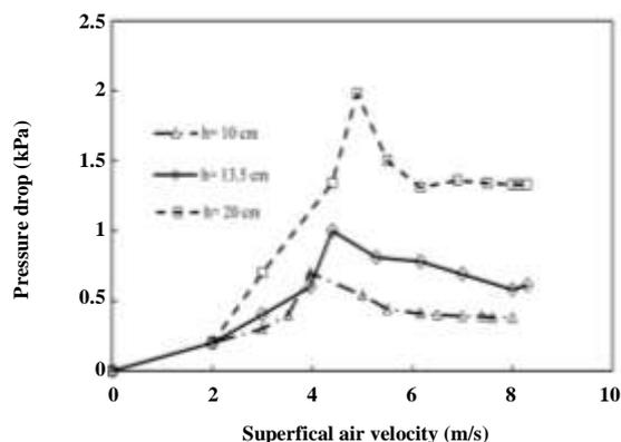
Fig. 3: Effects of static bed height on the pressure drop in binary sand particles. Jetsam rich system, sand (1): 1.77mm, 2650 kg/m<sup>3</sup>, 95%; sand (3): 0.356 mm, 2650 kg/m<sup>3</sup>, 5%, cone angle=30°.
