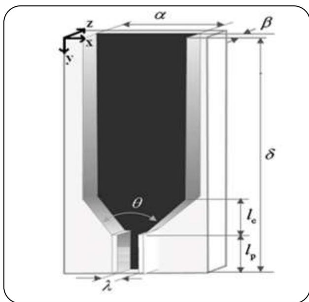
Fig. 1: Schematic of the spouted bed.
