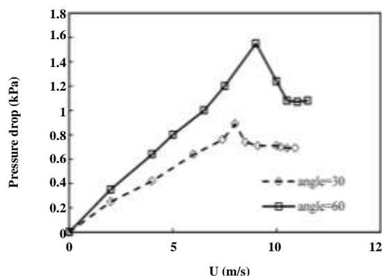
Fig. 6: Impact of cone angle on the pressure drop in the case of flotsam rich systems. Polyurethane: 380 kg/m<sup>3</sup>, 3.55 mm, 95%. Gypsum: 2700 kg/m<sup>3</sup>, 3.55 mm, 5%. Static bed height is  $h=40$  cm.
