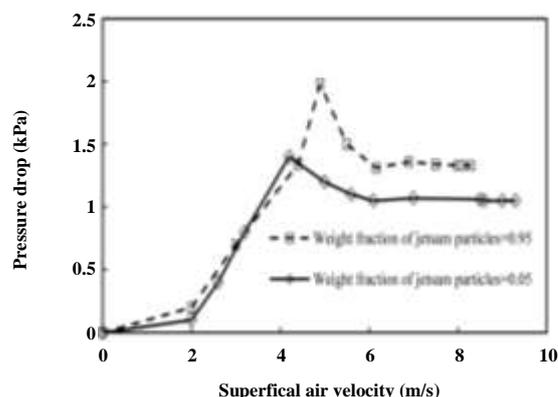
Fig. 4: Pressure drop profile in different binary mixture systems. Jetsam rich systems. (90% jetsam) and flotsam rich systems (5% jetsam). Sand (1): 1.77mm, 2650 kg/m<sup>3</sup>; sand (2): 0.575 mm, 2650 kg/m<sup>3</sup>. Static bed height, h= 20 cm, cone angle=30°.
