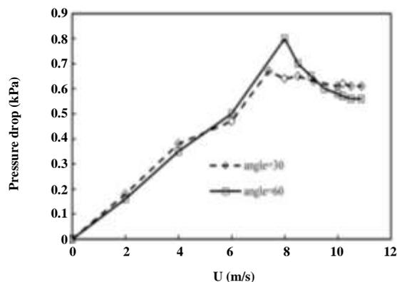
Fig. 5: Effects of cone angle on the variation of pressure drop against superficial gas velocity. Flotsam rich systems. Polyurethane: 380 kg/m<sup>3</sup>, 3.55 mm, 95%. Gypsum: 2700 kg/m<sup>3</sup>, 3.55 mm, 5%. Static bed height is  $h=20$  cm.
