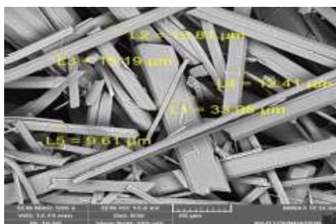
Fig. 6: The EDX and SEM analysis results; a) EDX and b, c) SEM of the crystals of W2.
