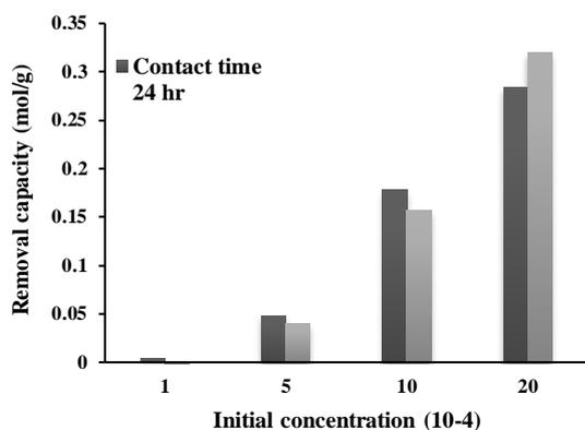
Fig. 9: Concentration of dye on the removal capacity when the contact time is 24 and 48 hr.
