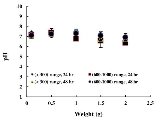
**Fig. 6:** pH values of samples of secondary metabolites compounds extracts produced from bio-waste at mesh sizes (< 300 and 600-1000)  $\mu\text{m}$ , weight of bio-waste (0.1, 0.5, 1, 1.5 and 2) g and contact time (24 and 48) hr in 25 mL D.W.
