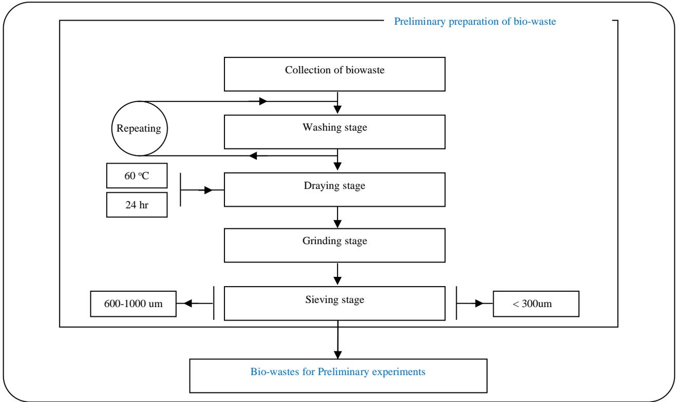
Fig. 1: A general layout of the preparation of the suggested adsorbents materials as preliminary preparation stages.
