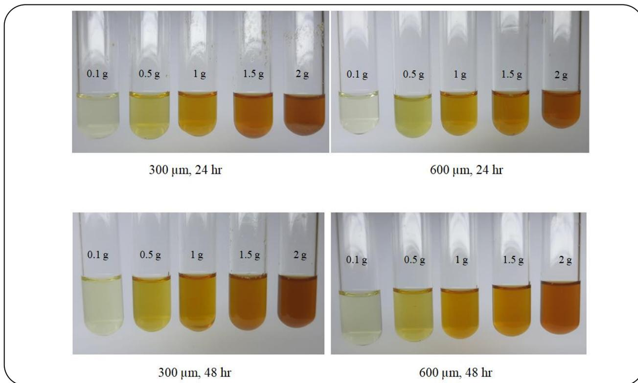
**Fig. 5:** Samples of secondary metabolites compounds extracts produced from bio-waste of biowaste at mesh sizes (< 300 and 600-1000)  $\mu\text{m}$ , weight of bio-waste (0.1, 0.5, 1, 1.5 and 2) g and contact time (24 and 48) hr in 25 mL D.W.
