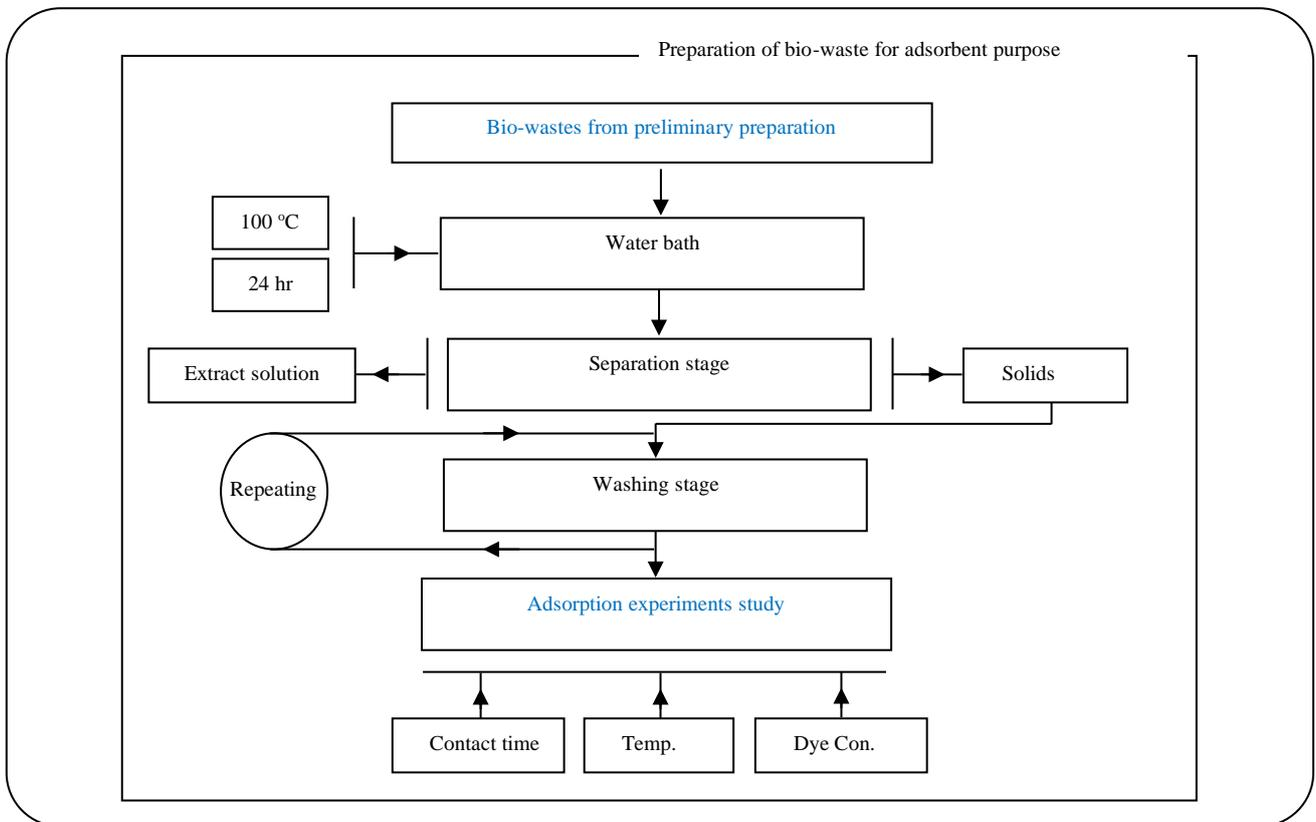
Fig. 2: A general layout of the thermal treatment as preparation stages of the suggested adsorbents materials.
