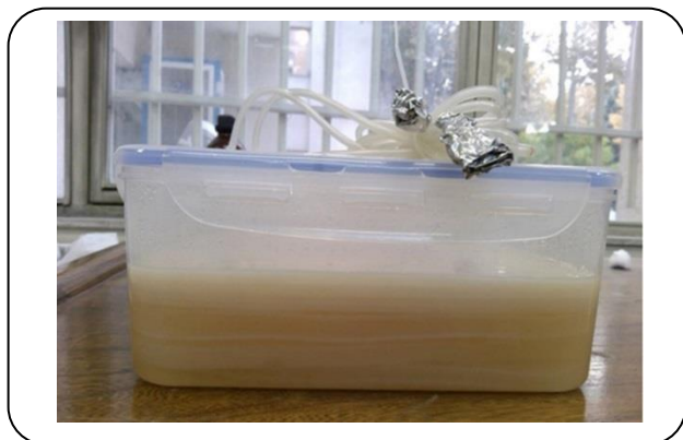
Fig. 2. BC production from Acetobacter xylinum in repeated static batch culture after 3 cycles.
