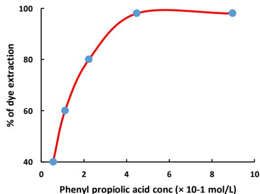
Fig. 4: Effect of carrier concentration (feed 25 mL of 50 mg/L of dye at  $\text{pH} 7 \pm 0.1$ , the volume of organic phase 25 mL, equilibration time 3 min).
