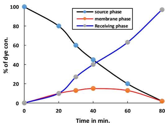
Fig. 8: Effect of time (volume of source phase 260 mL of 50 mg/L of dye at pH  $7 \pm 0,1$  carrier concentration  $4.48 \times 10^{-1}$  mol/L, volume of receiving phase 260 mL of 1N H<sub>2</sub>SO<sub>4</sub> and rate of stirring 400rpm).
