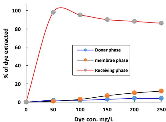
Fig. 7: Effect of dye concentration (volume of source phase 260 mL of different concentration of dye at pH  $7 \pm 0,1$  carrier concentration  $4.48 \times 10^{-1}$  mol/L, volume of receiving phase 260 mL of 1N H<sub>2</sub>SO<sub>4</sub>, rate of stirring 400rpm and effect of time 70 min).
