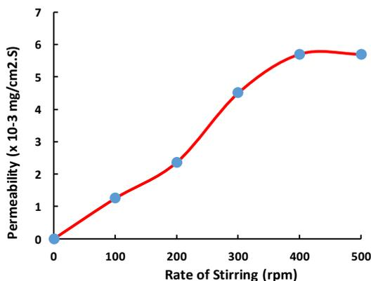
**Fig. 5: Effect of stirring speed (volume of source phase 260 mL of 50mg/L of dye at pH 7 ± 0.1, carrier concentration 4.48 × 10<sup>-1</sup> mol/L, volume of receiving phase 260 mL of 1N H<sub>2</sub>SO<sub>4</sub>, and effect of time 70 min).**
