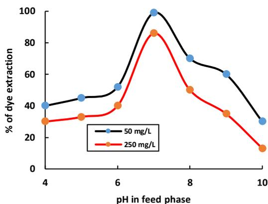
Fig. 5: Effect of pH of feed phase (volume of source phase 260 mL of 50 mg/L and 250 mg/L of dye at various, pH carrier concentration  $4.48 \times 10^{-1}$  mol/L, volume of receiving phase 260 mL of 1 N H<sub>2</sub>SO<sub>4</sub>, rate of stirring 400 rpm and effect of time 70 min. .
