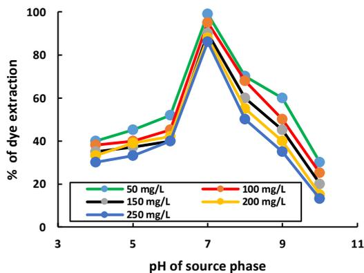
Fig. 3: Effect of pH in source phase (volume of feed 25 mL, carrier concentration  $4.48 \times 10^{-1}$  mol/L, volume of organic phase 25 ml and equilibration time 3 min).
