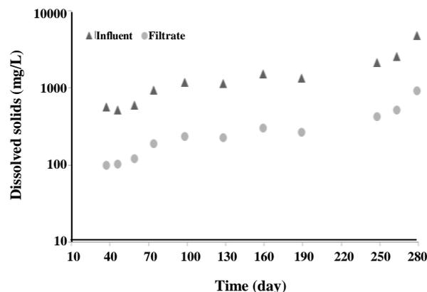
Fig. 5: Trend of Dissolved Solids in influent and filtrate of the membrane bioreactor.
