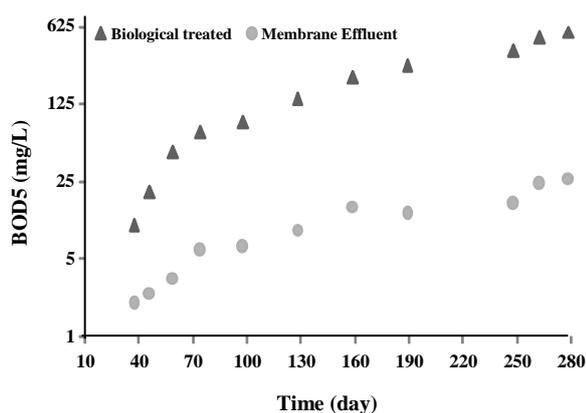
Fig. 2: Trend of BOD<sub>5</sub> concentration in biological and membrane effluent.
