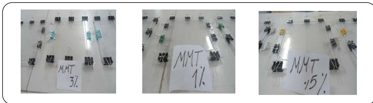
Fig. 1: Prepared CMC/PVA composite films based on different loadings of nanoclay.
