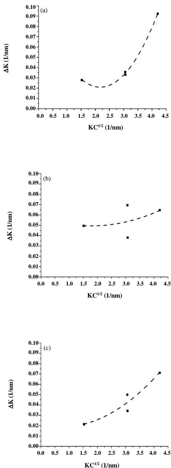
Fig. 3: Modified Williamson-Hall plot ( $\Delta K$  versus  $KC^{1/2}$ ) of annealed and SSEed specimens.
