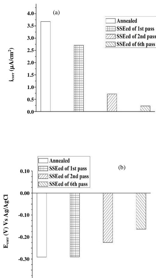
Fig. 7: Corrosion currents (a) and corrosion potentials (b) of annealed and SSEd samples.
