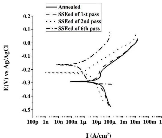
Fig. 6: Tafel plots of annealed and SSEd samples.
