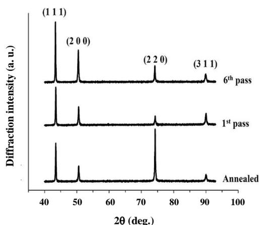
Fig. 2: XRD patterns of annealed and SSEed samples.
