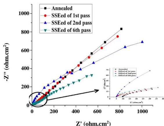
Fig. 4: Nyquist plots of annealed and SSEEd samples.
