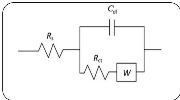
Fig. 5: The equivalent circuit used for fitting the experimental EIS data.
