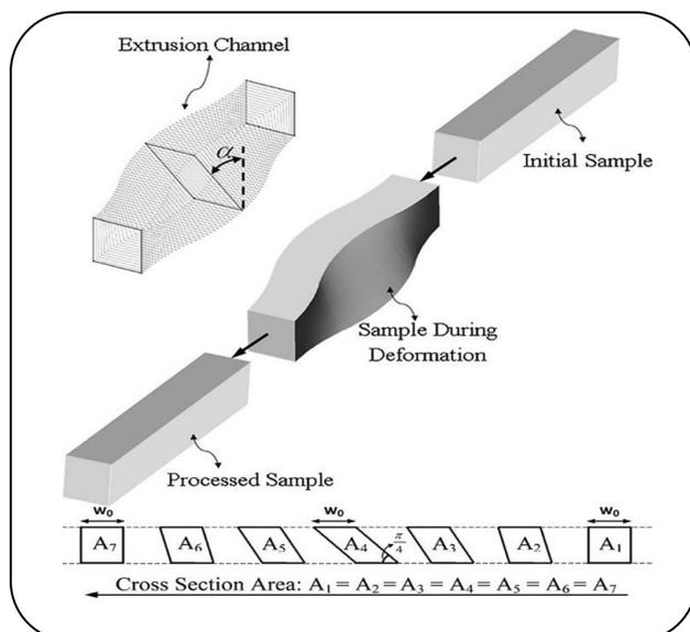
Fig.1. Schematic presentation of Simple Shear Extrusion process and the geometry of extrusion channel in the die [2].
