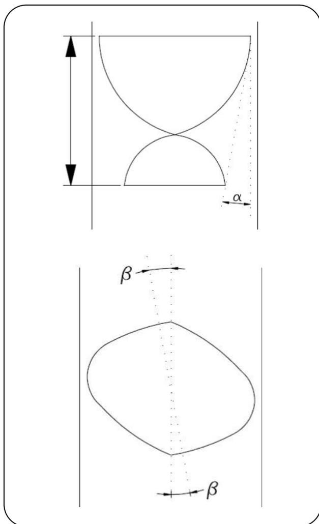
Fig. 3: The Fluid Flow Pattern in the Tubular Reactor with Helical Element (Parabolic Path/Exponential Path).
