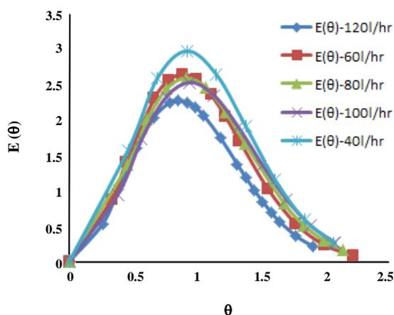
**Fig. 5: Typical RTD curves at different volumetric flow rate.**
