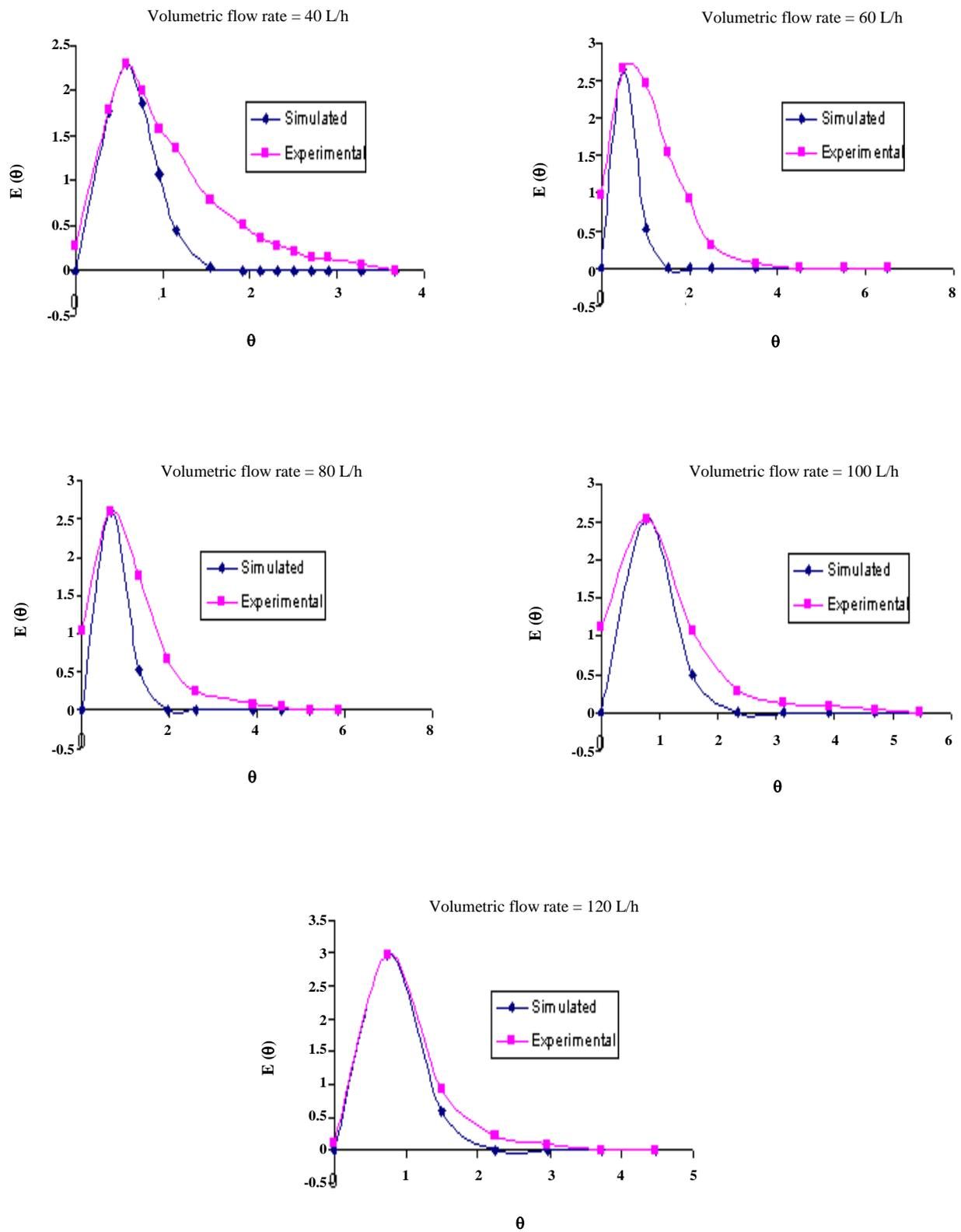
Fig. 4: Comparison of RTD curves between simulations and experimental data.
