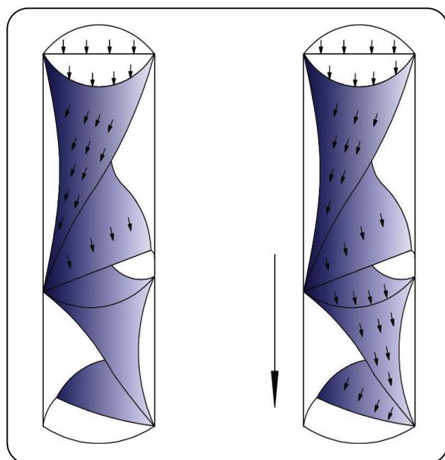
**Fig. 2: Flow of fluid in the tubular reactor with helical element.**
