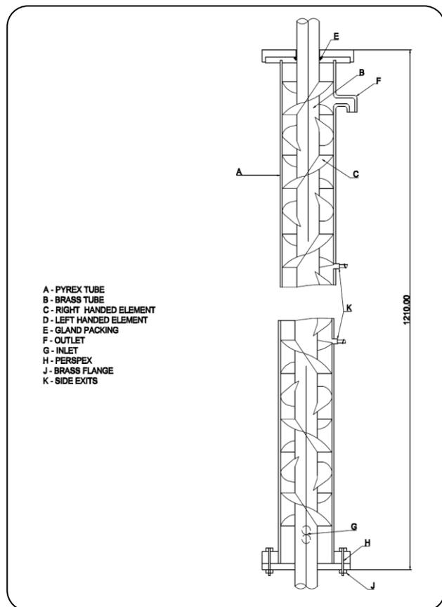
**Fig.. 1. Tubular flow reactor with helical mixing elements with increasing flow rate.**
