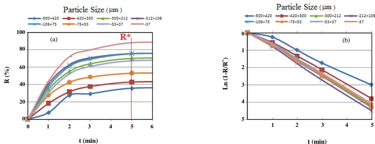
Fig. 1: Calculation of flotation rate constant ( $k$ ) based on  $R^*$  for  $S_b = 28.23$  l/s.
