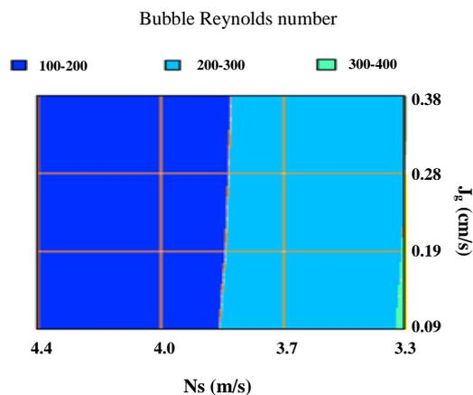
Fig. 5: Bubble Reynolds number in different peripheral impeller speeds and superficial gas velocity.
