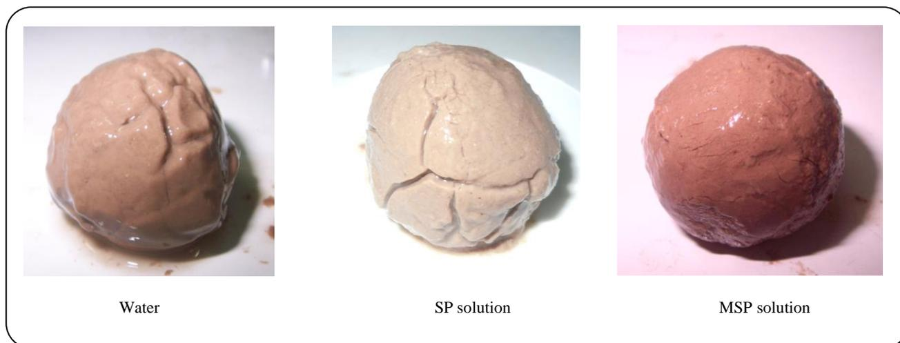
Fig. 4: The status of mud balls immersed in different fluids for 36 h.
