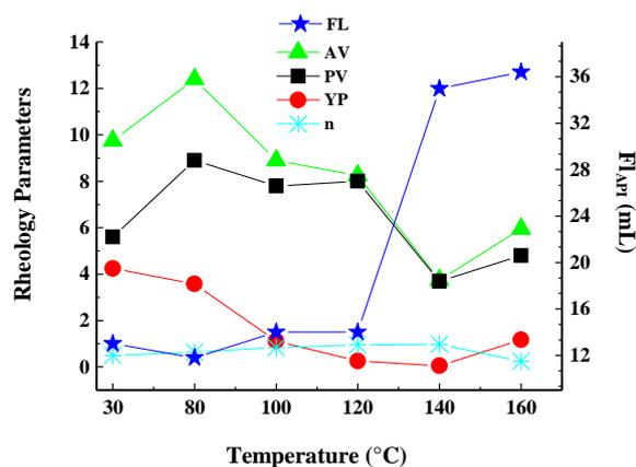
**Fig. 2: Effect of temperature on rheology property of MSP modified drilling fluids.**
