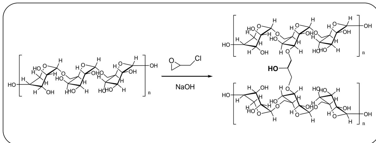
Fig. 1: Reaction of SP gum with epichlorohydrin.
