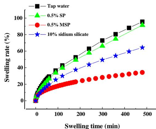
**Fig. 3: The swelling rate of the clay in different solutions.**
