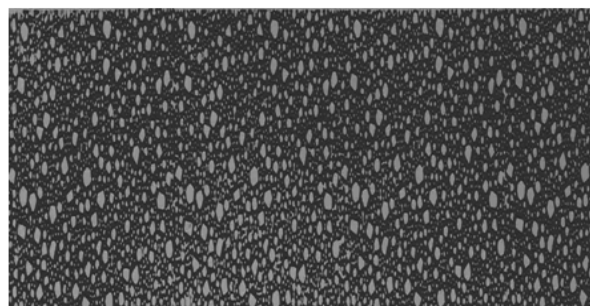
Fig. 1: Micromodel pattern which is fully saturated with colored blue water.
