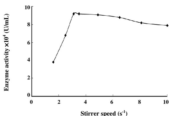
Fig. 5: Effect of stirrer speed on extraction of lipoxygenase-1 in scaled-up stirred vessel.
