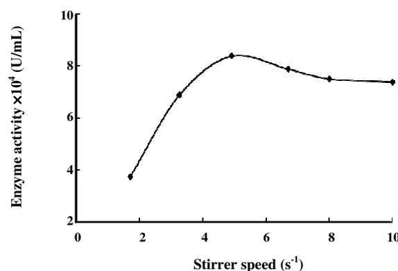
Fig. 3: Effect of stirrer speed on extraction of lipoxygenase-1.
