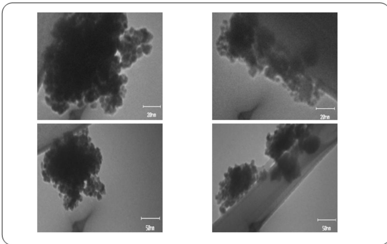
*Fig. 5: TEM image of the as- prepared ZrO<sub>2</sub> nanoparticles (Sample 2).*
