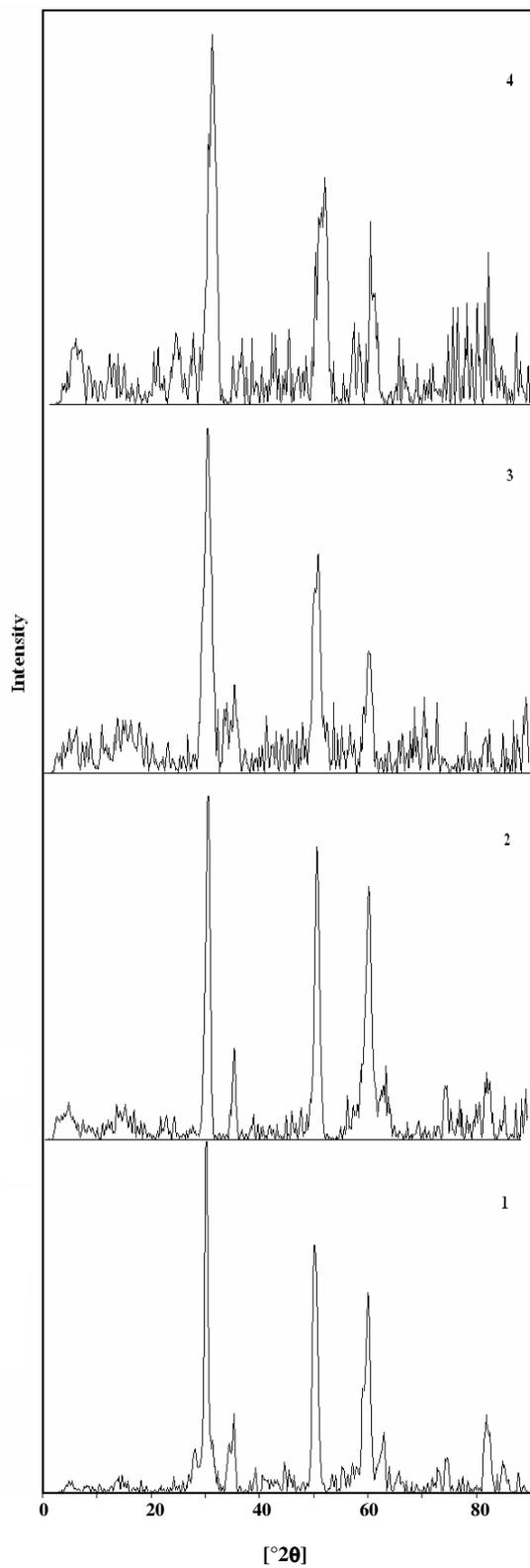
Fig. 1: XRD patterns of the as-prepared ZrO<sub>2</sub> nanoparticles (Samples 1,2,3,4).
