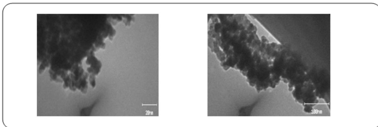
*Fig. 6: TEM image of the as- prepared ZrO<sub>2</sub> nanoparticles (Sample 7).*
