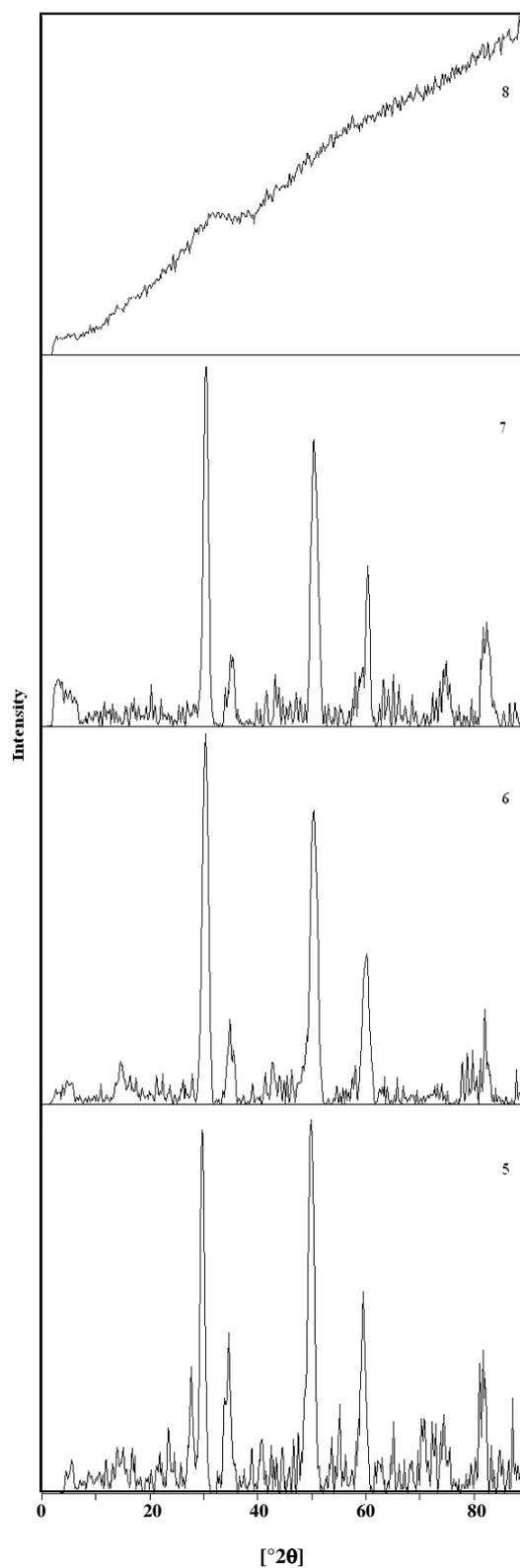
Fig. 2: XRD patterns of the as-prepared ZrO<sub>2</sub> nanoparticles (Samples 5,6,7,8).
