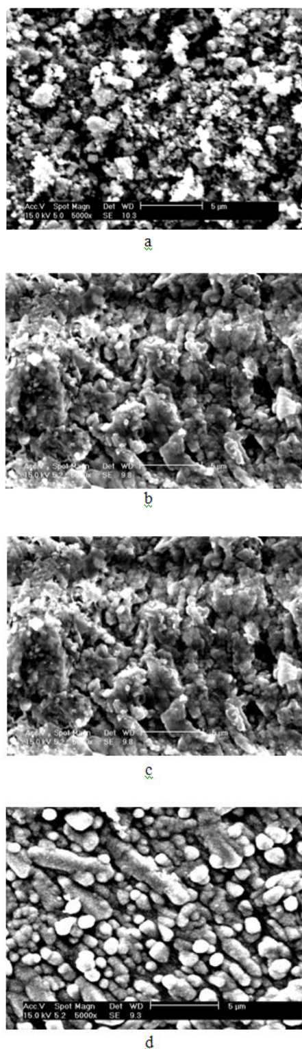
Fig. 8: SEM images dip coated doped \text{SnO}_2 film with different antimony concentrations (g/lit) at 5 dips and 550^\circ\text{C} : a) 8.52, b) 17.04, c) 25.6, d) 34.12.
